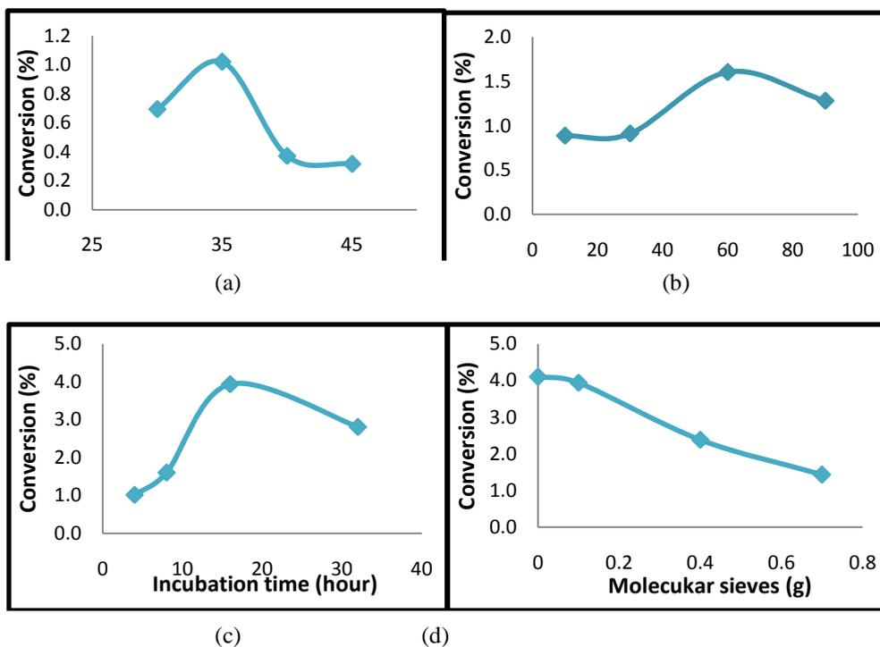
Figure 2. The effect of temperature (a), the ratio of the substrate G:FA (b), incubation time (c) and molecular sieve added (d) to the percent conversion of glucose-fatty acid esters.
