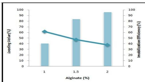
Figure 1. The effect of alginate concentration to the loading value (%) and the immobilization efficiency (%). The loading value (bar) and the immobilization efficiency (◆).
