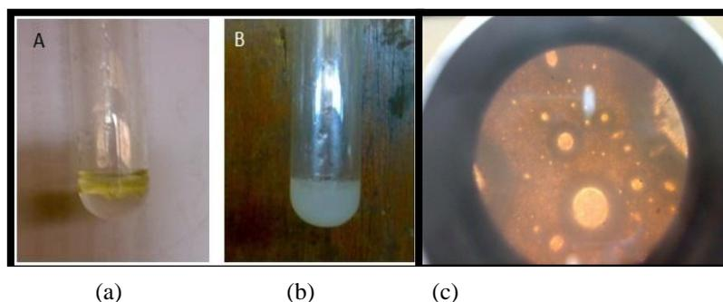
Figure 3. Simple emulsion test results prior to the addition of the reaction product (a) after addition of the reaction product (b) and the observation of emulsions formed with a microscope is known that the emulsion formed is an emulsion of oil in water (o/w).
