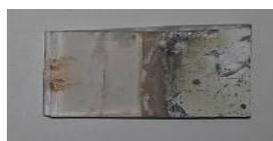
**Fig.4** The synthesis of Cu<sub>2</sub>O-ZnO/FTO
