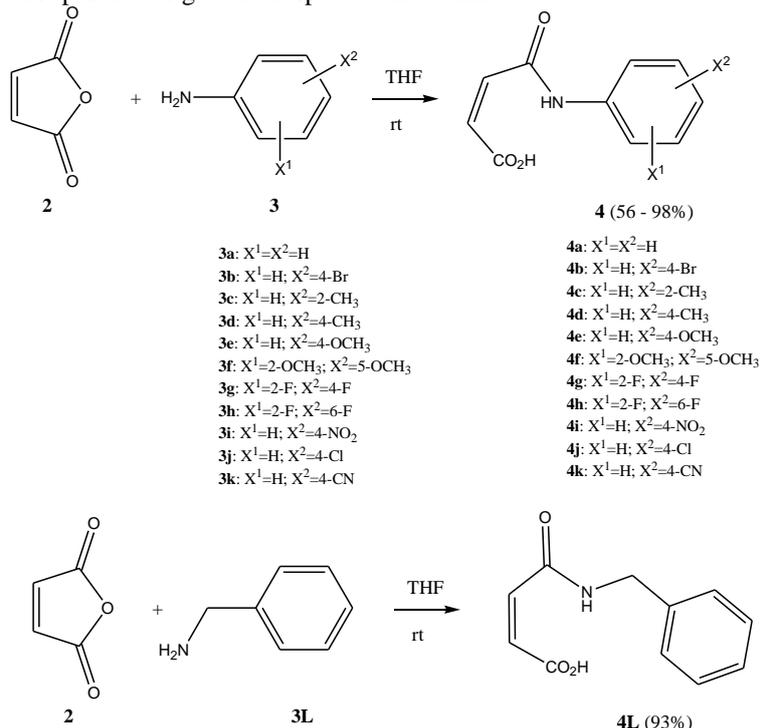
**Scheme 1.** Known synthesis of maleanilic acids (**4**) from maleic anhydride (**2**) and anilines (**3**).
