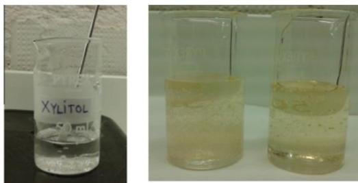
Figure no 2. Discoloration of the xylitol solution after heating<sup>9</sup>
