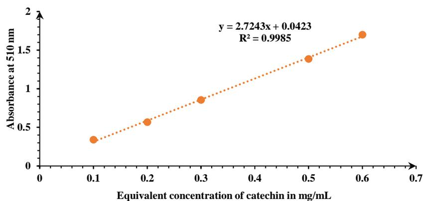
Figure 4: Calibration curve for catechin
