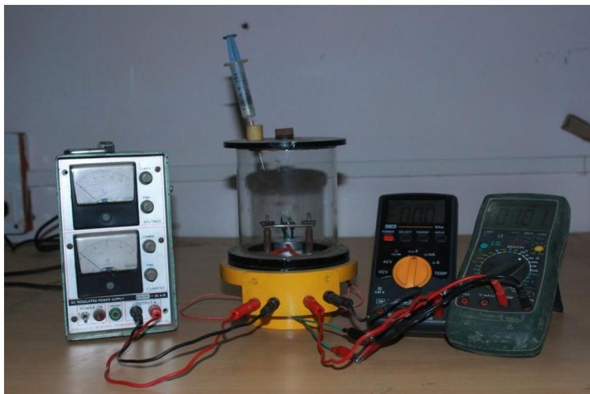
**Figure 2: Photograph of the proposed gas sensor setup.**
