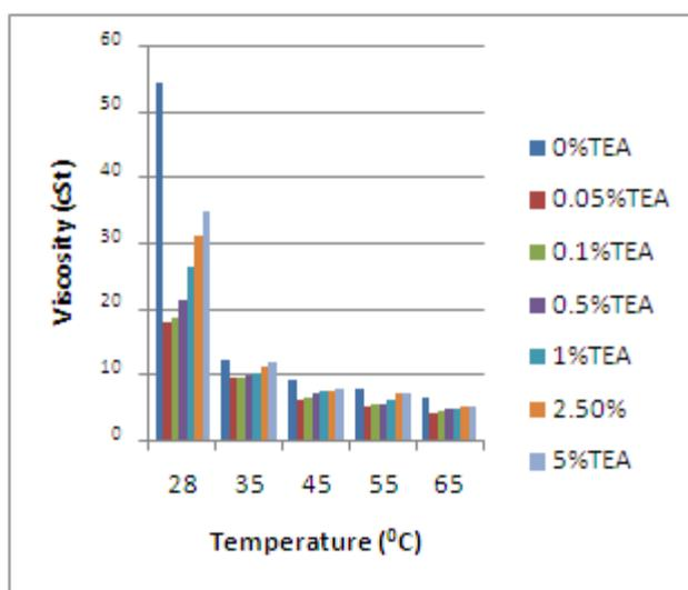
**Figure1: Chart of proportions of TEA in crude oil and its viscosity**
