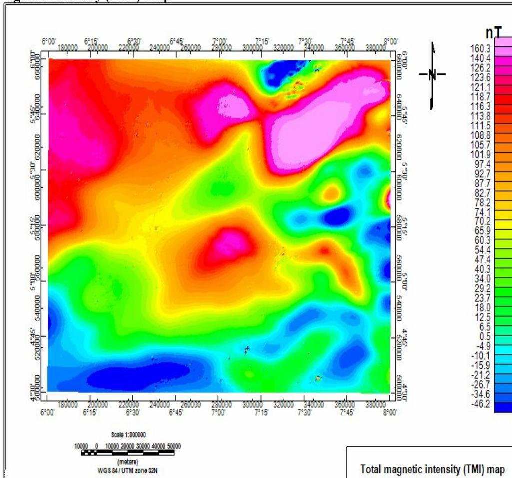
**Figure 2: Result of Total Magnetic Intensity Map**
