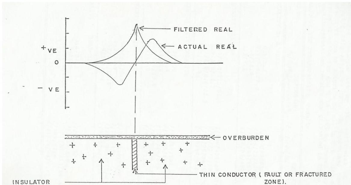
Fig. 2 Theoretical EM (VLF) response over a vertical dipping conductive sheet (fault, fractured, fissured zone or lithological contact)
