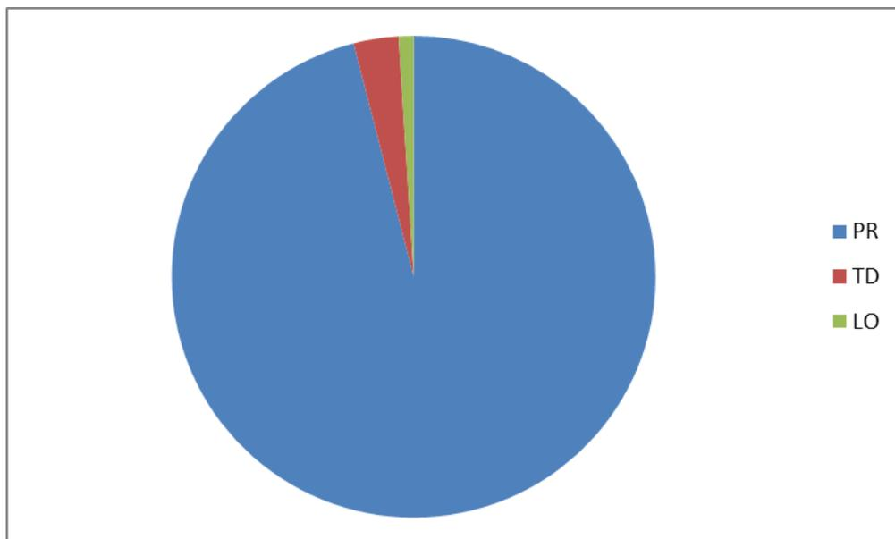
**Figure 12.** Percentage of bits dull graded in terms of pull out of hole.
