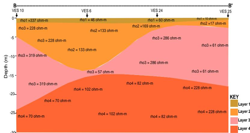
Fig. 11 Resistivity profile along BB'
