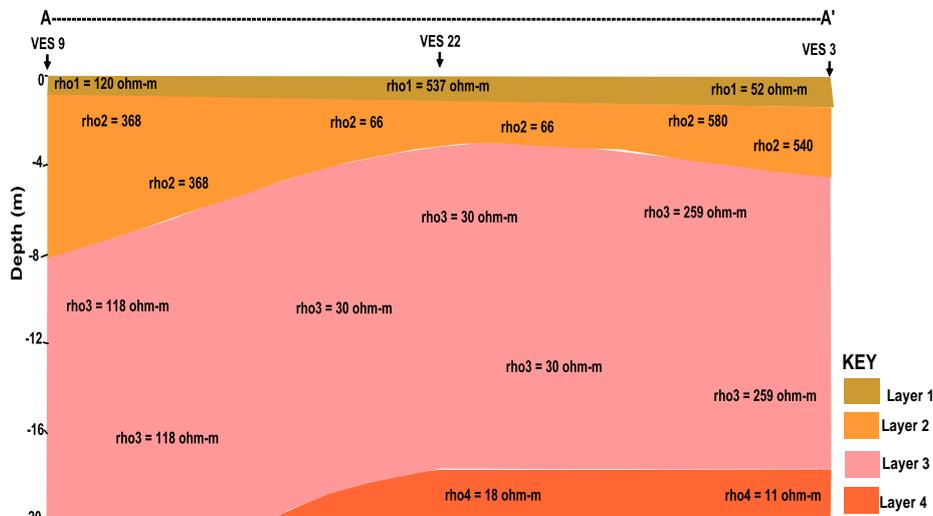
Fig. 10 Resistivity profile along AA'
