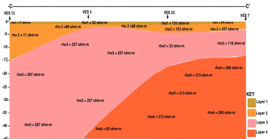
Fig. 12 Resistivity profile along CC'
