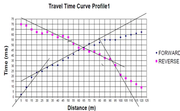
**Figure 3:** Forward and Reverse Profile Plot, Profile 1
