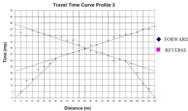
Figure 7: Forward and reverse profile plot, profile 3
