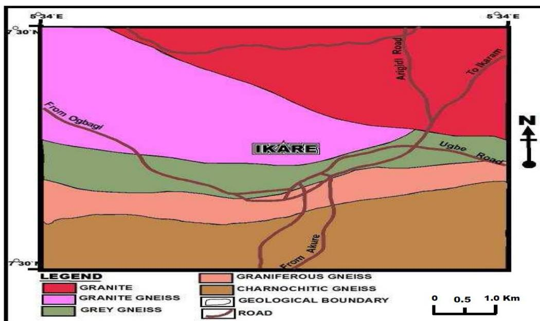
**Fig. 2:** Geological Map of Ikare-Akoko (Extracted from Geological map of Ondo State).
