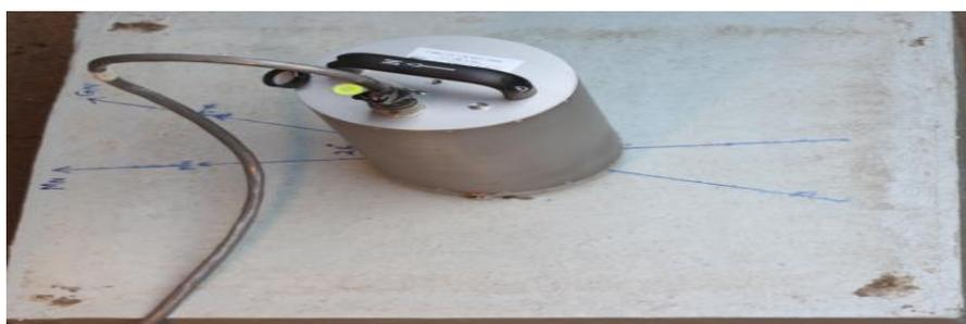
Figure 3. Installation of Broadband Seismometer inside the Seismic Vault.
