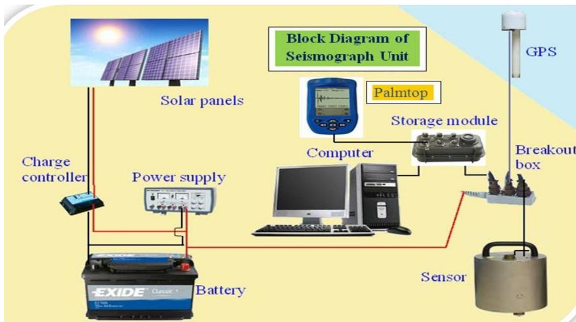
Figure 4. Block diagram of Seismograph Setup at Maitri Antarctica
