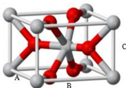
**Figure 3.** The model of the unit cell of the crystal rutile SnO<sub>2</sub>
