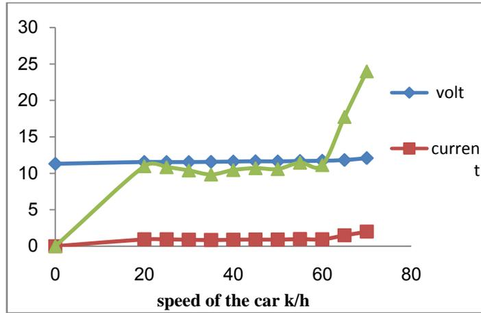
Figure no2: The speed against the volt, current and power for second fan
