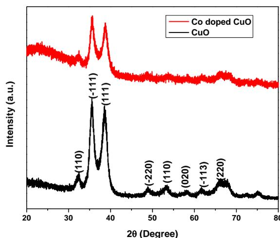
Figure 1. XRD pattern of pure and Co doped CuO thin films.
