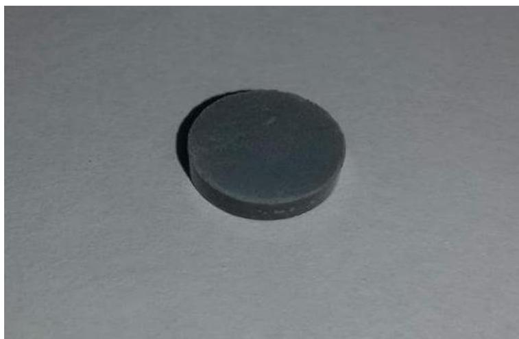
**Fig.2.2:** Disk shaped pellet of Cu doped ZnO sample sintered at  $600^\circ C$  for 8 hours.
