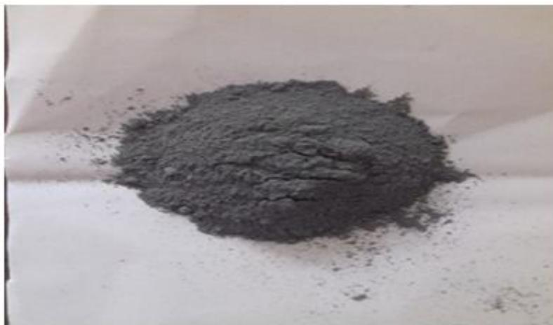
**Fig.2.1:** Powder sample of Cu doped ZnO calcined at  $500^\circ C$  for 12 hours.
