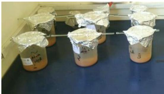
Figure 1: Photographs of long term immersion corrosion test
