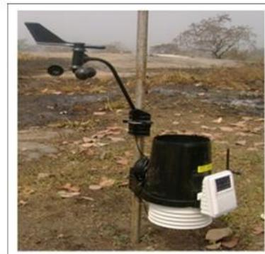
**Fig 1.3:** The Integrated Sensor Suite (ISS) on site at Awka
