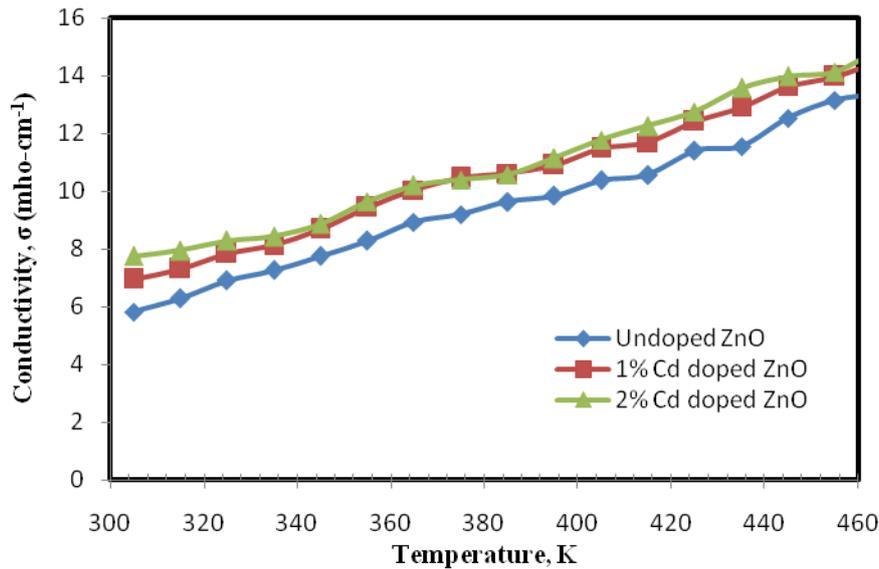
**Fig 6:** Variation of conductivity with temperature for undoped and Cd:ZnO thin films
