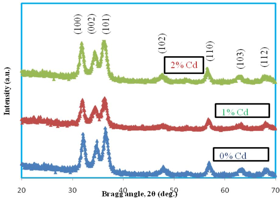
Fig. 1: X-ray diffraction pattern for undoped and Cd:ZnO thin films.
