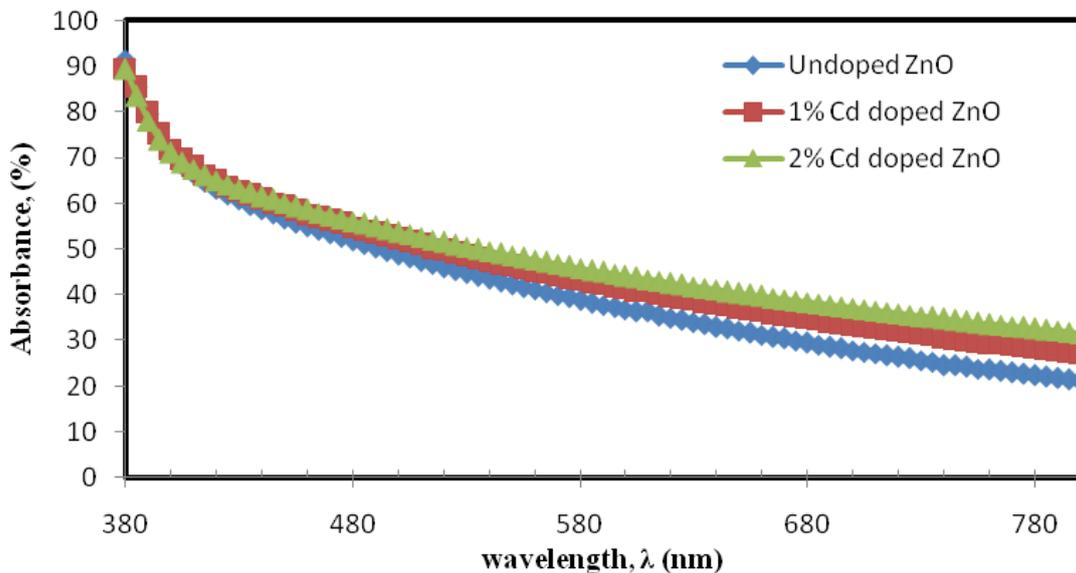
Fig. 3: Variation of optical absorbance with wavelength for undoped and Cd:ZnO thin films.
