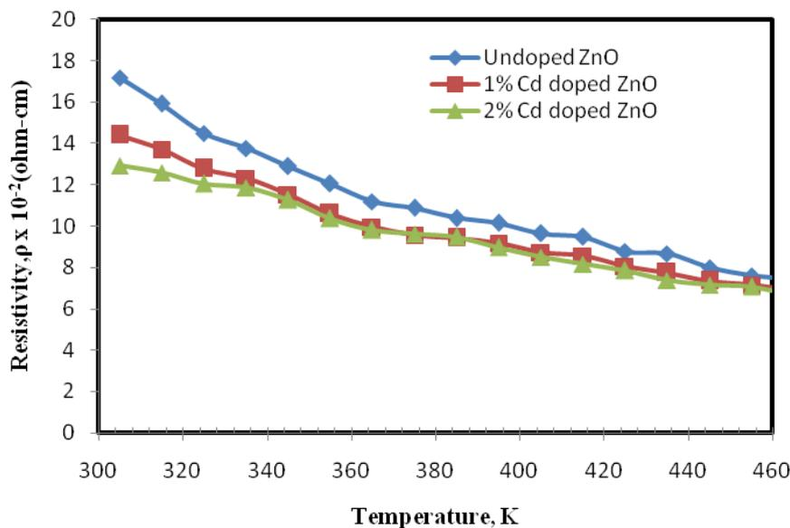
Fig 5: Variation of resistivity with temperature for undoped and Cd:ZnO thin films.
