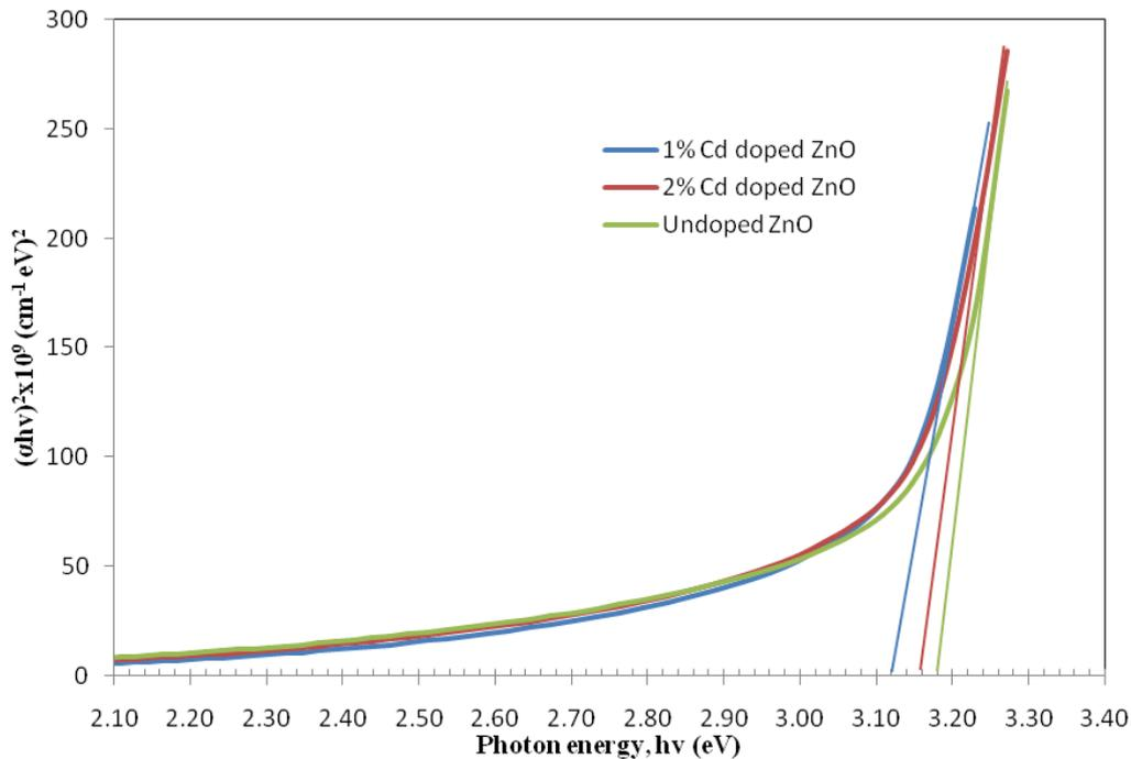
Fig. 4: Variation of  $(\alpha h\nu)^2$  with photon energy for undoped and Cd:ZnO thin films.
