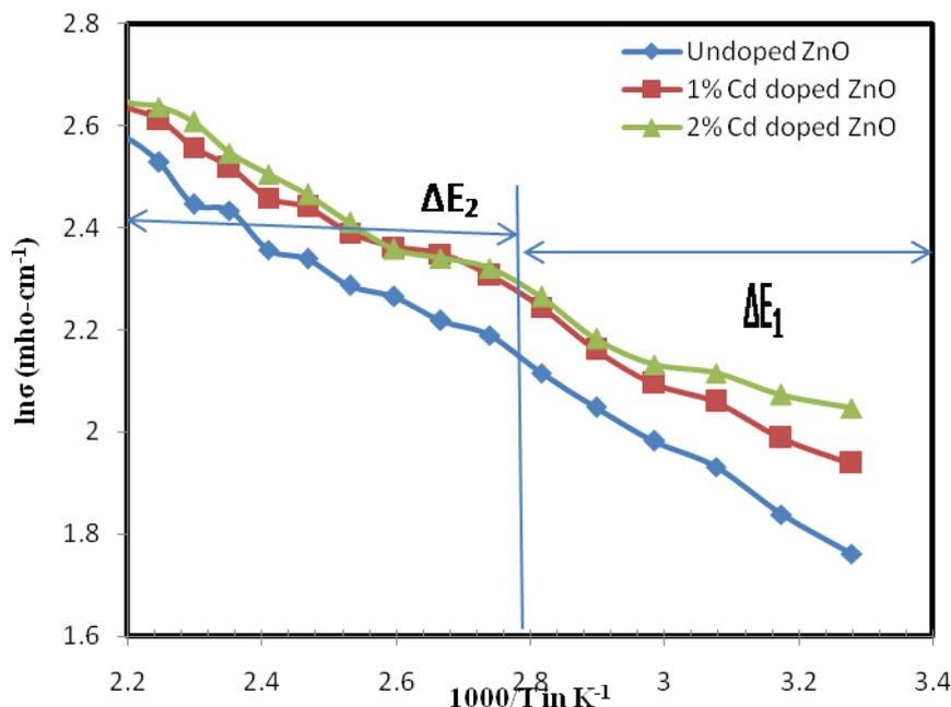
**Fig 7:** Variation of  $\ln\sigma$  with  $1000/T$  for undoped and Cd:ZnO thin films.
