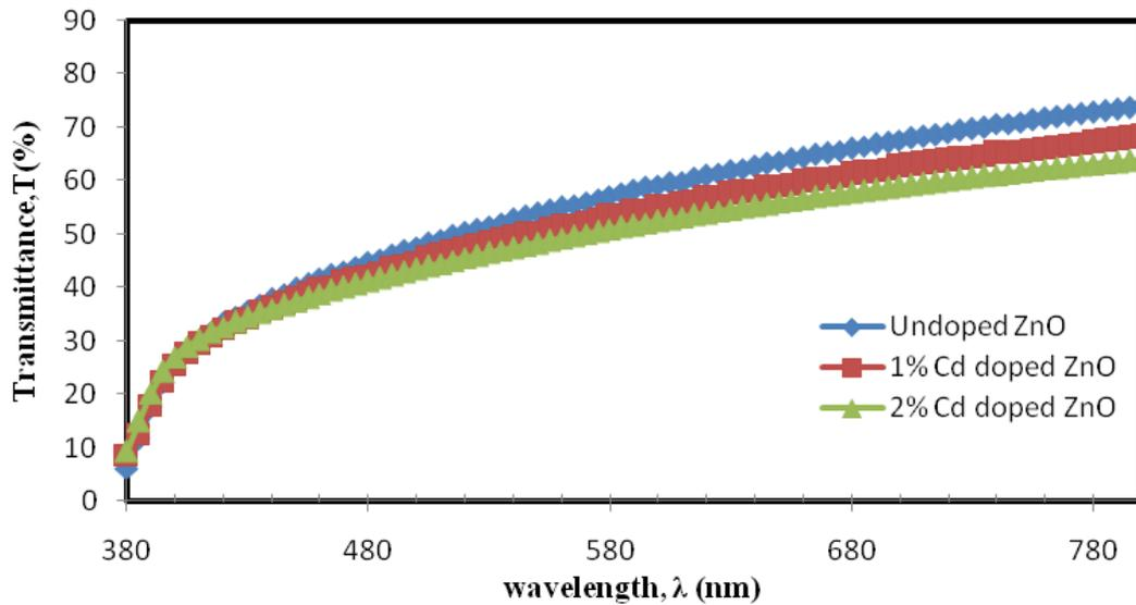
Fig. 2: Variation of optical transmittance with wavelength for undoped and Cd:ZnO thin films.
