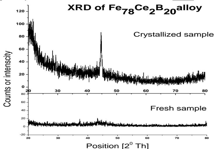
**Figure 3** XRD pattern of amorphous and crystallized  $Fe_{78}Ce_2B_{20}$  alloy recorded at room temperature.
