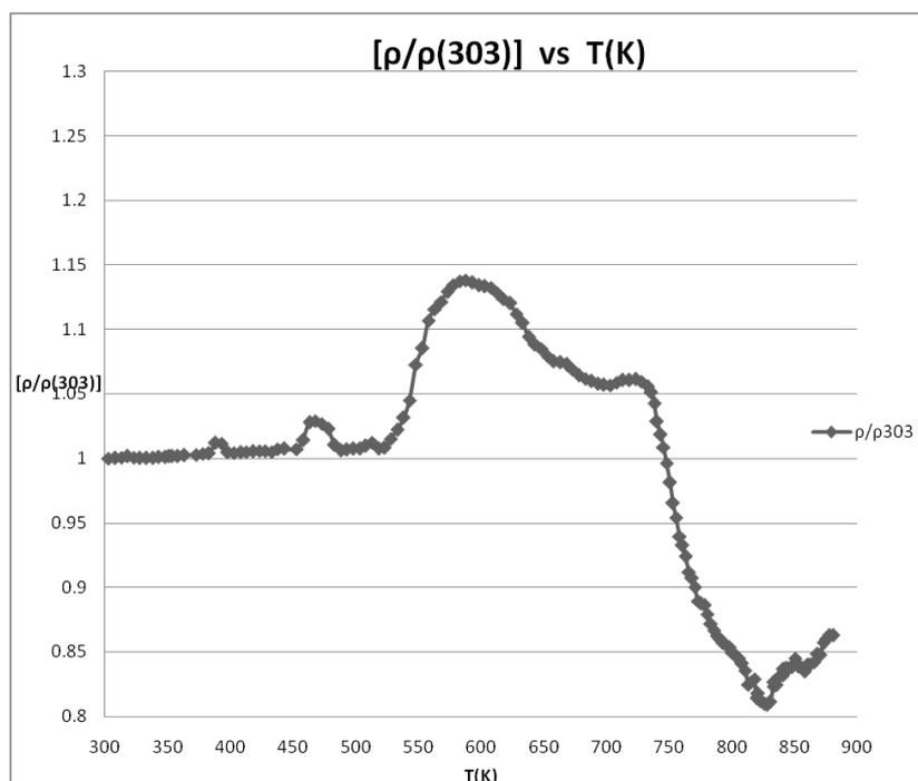
**Figure 2:** Resistivity Ratio,  $\rho/\rho_{(303)}$  versus Temperature (T) of amorphous  $Fe_{78}Ce_2B_{20}$  alloy
