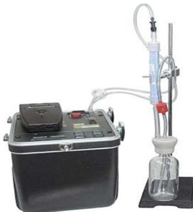
**Fig 2:** Arrangement of apparatus for measuring radon content in the carbonated drinks.
