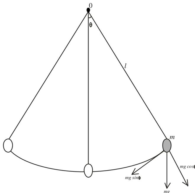
Figure 1: Simple Pendulum [8]
