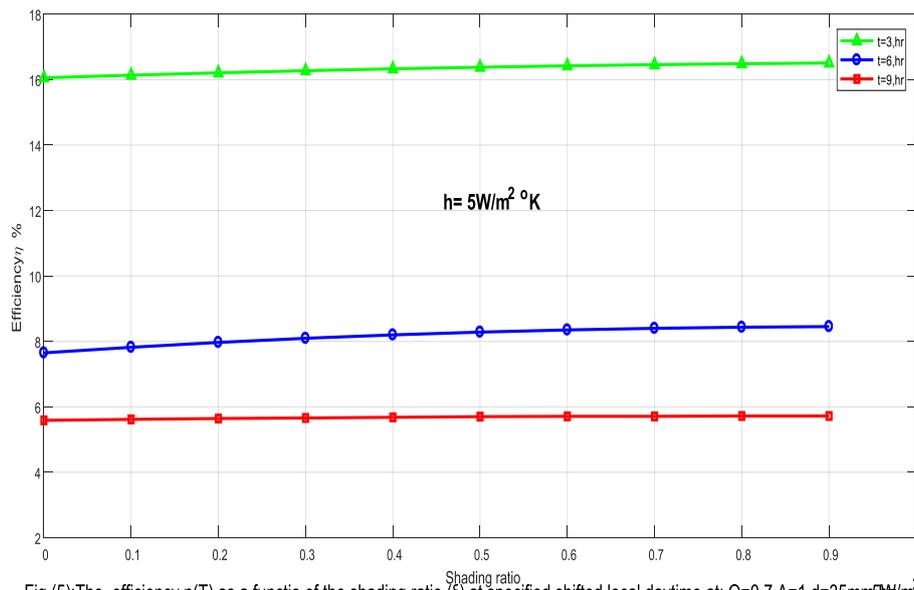
Fig.(5):The efficiency  $\eta(T)$  as a function of the shading ratio ( $\xi$ ) at specified shifted local daytime at:  $Q=0.7, A=1, d=35 \text{ mm}, h=5 \text{ W/m}^2 \text{ }^\circ\text{K}$
