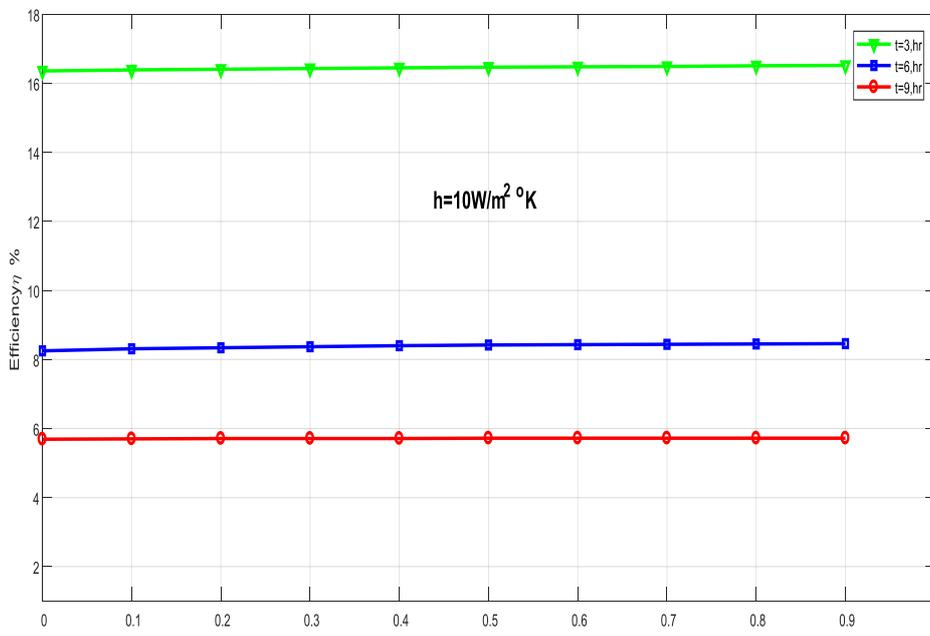
Fig.(6):The efficiency  $\eta(T)$  as a function of the shading ratio ( $\xi$ ) at specified shifted local daytime at:  $Q=0.7, A=1, d=35 \text{ mm}, h=10 \text{ W/m}^2 \text{ }^\circ\text{K}$
