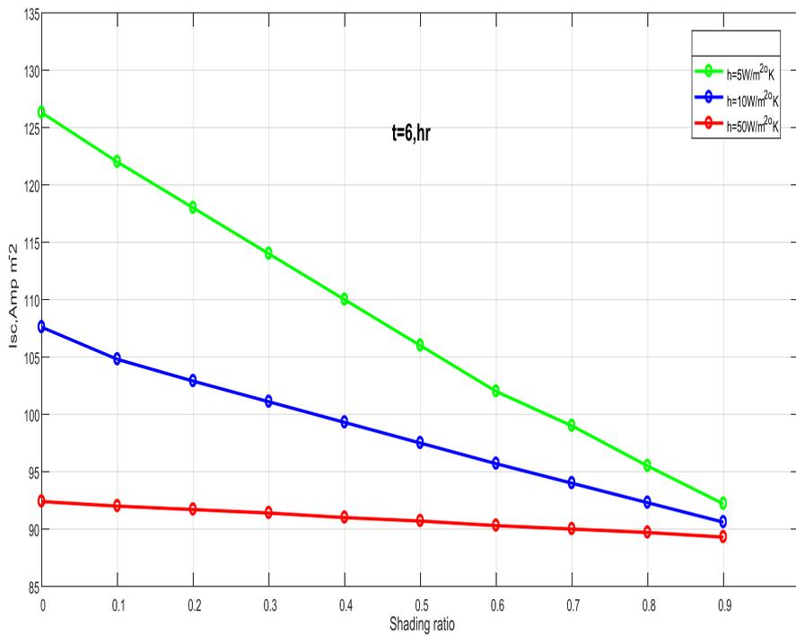
Fig.(10):The relation between the  $I_{sc}$  with different shading ratio at:( $t=6\text{hr}$ ,  $Q=0.7$ ,  $A=1$ ,  $d=35\text{mm}$ )
