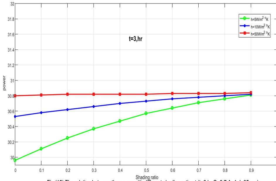
Fig.(15):The relation between the power with different shading ratio at:(t=3,hr,Q=0.7,A=1,d=35mm)
