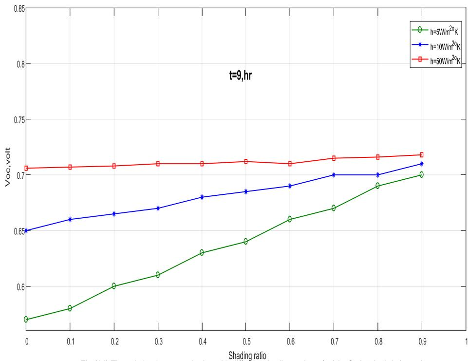
Fig.(14):The relation between the Voc with different shading ratio at:(t=9,hr,Q=0.7,A=1,d=35mm)
