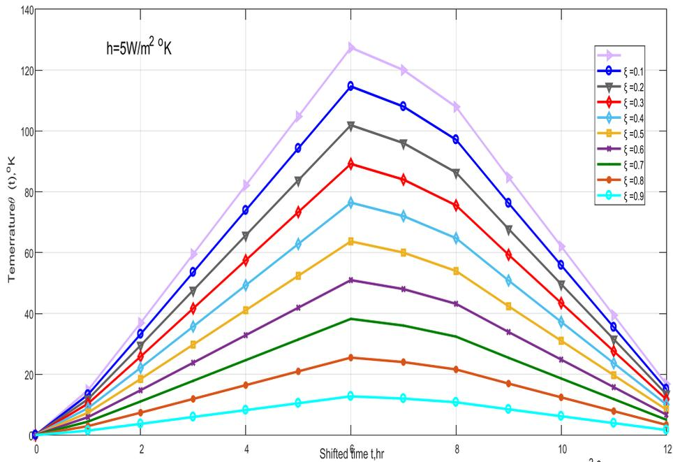
Fig(2): The relation between solar cell temperature according to (Eq.9 and Eq.10 ) and local solar time at different Shading levels for ( $h=5 \text{ W/m}^2 \text{ }^{\circ}\text{K}$ ,  $d=.035\text{m}$ ,  $A=1$ )
