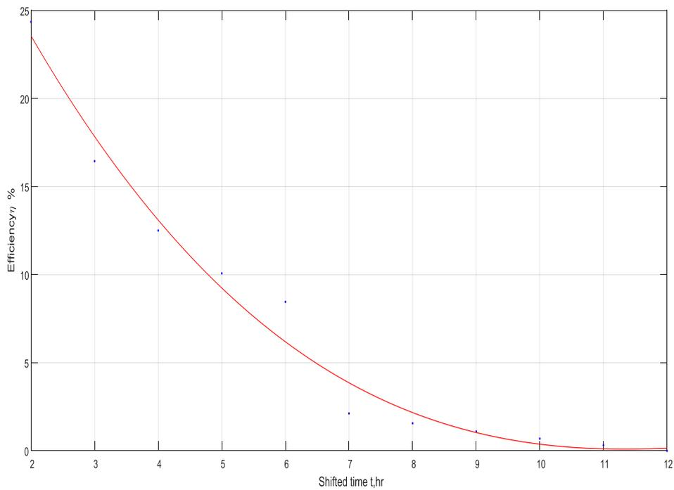
Fig.(8):The relation between the efficiency and local shifted solar time at constant shading at: ( $h=10W/m^2K, Q=0.7, d=35mm, A=1, \xi=0.4$ )
