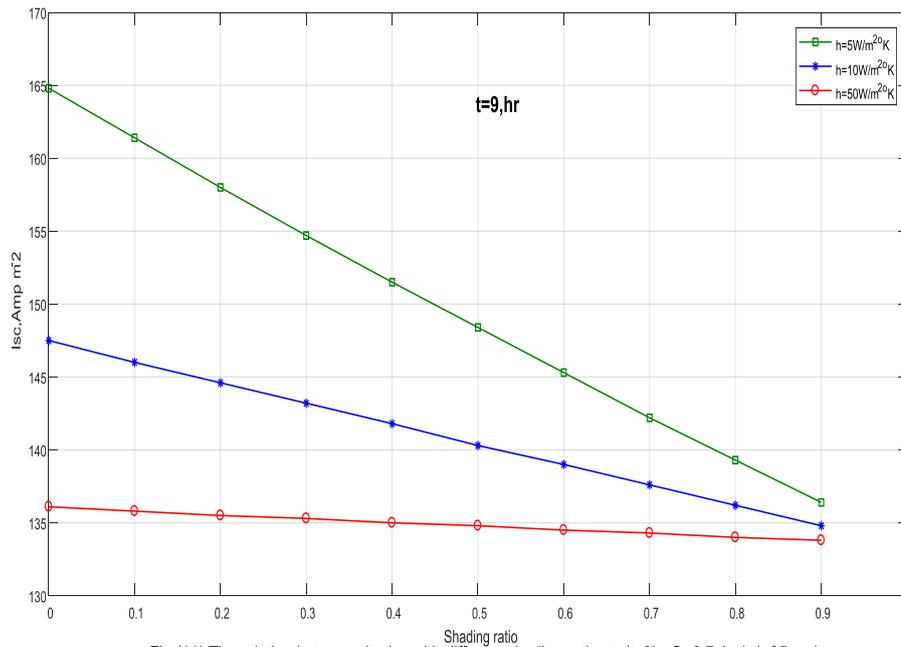
Fig.(11):The relation between the Isc with different shading ratio at: (t=9hr,Q=0.7,A=1,d=35mm)
