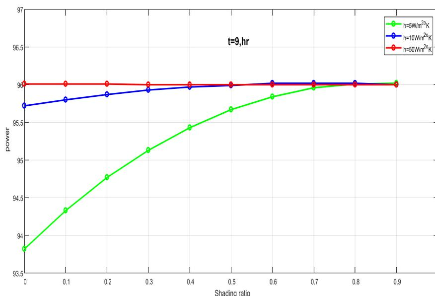
Fig.(17):The relation between the power with different shading ratio at:(t=9,hr,Q=0.7,A=1,d=35mm)
