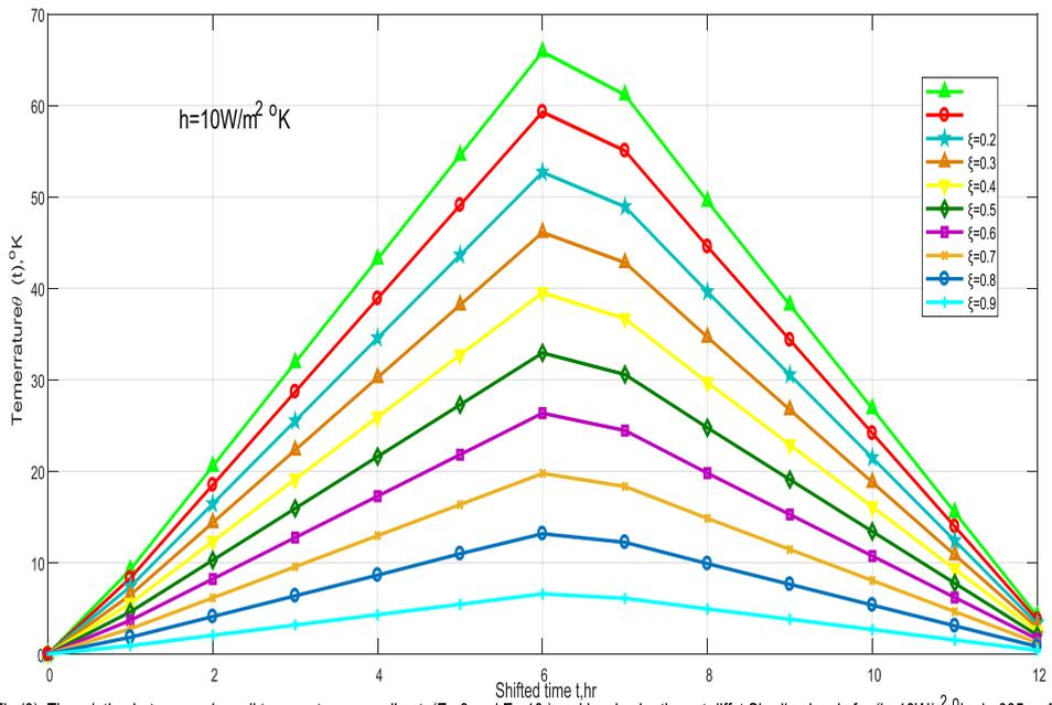
Fig.(3): The relation between solar cell temperature according to (Eq.9 and Eq.10 ) and local solar time at different Shading levels for ( $h=10 \text{ W/m}^2 \text{ }^{\circ}\text{K}$ ,  $d=.035\text{m}$ ,  $A=1$ )
