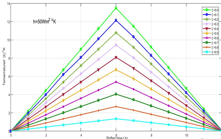
Fig.(4):The relation between solar cell temperature according to(Eq.9 and Eq.10)and local shifted solar time at different Shading levels for (h=50W/m<sup>2</sup> °K, d=35mm, A=1)
