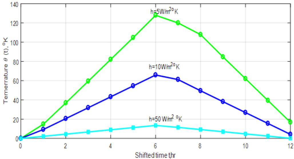
Fig.(1):The relation between the unshaded solar cell temperature and local shifted solar day time for different cooling conditions)
