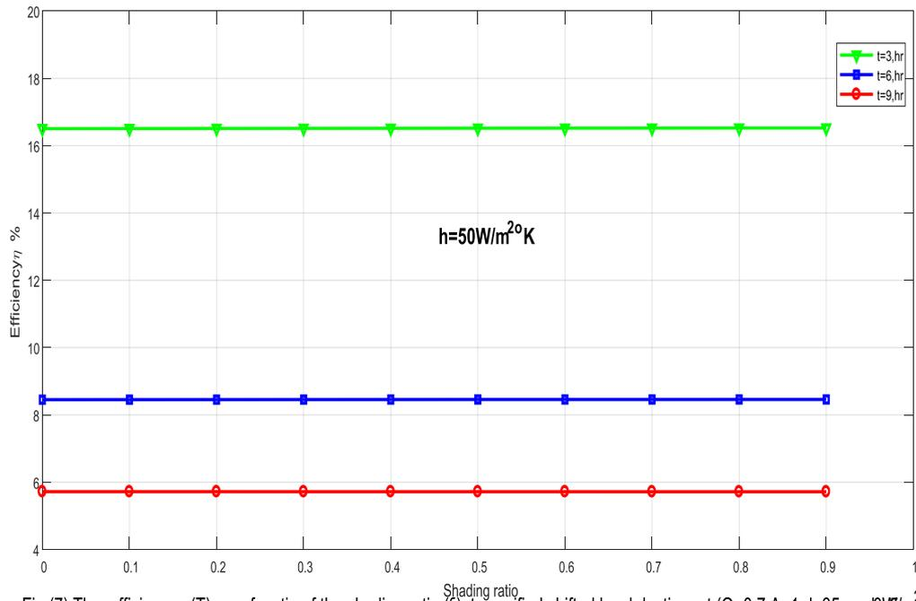
Fig.(7):The efficiency  $\eta(T)$  as a function of the shading ratio ( $\xi$ ) at specified shifted local daytime at: ( $Q=0.7, A=1, d=35mm, h=50W/m^2k^0$ )
