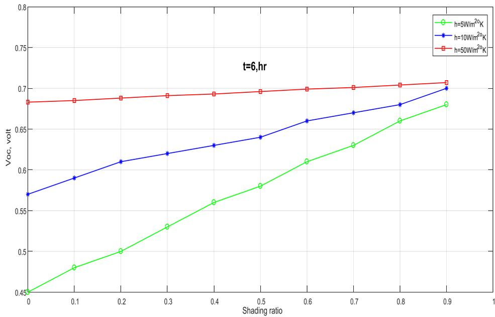
Fig.(13):The relation between the Voc with different shading ratio at:(t=6,hr,Q=0.7,A=1,d=35mm)
