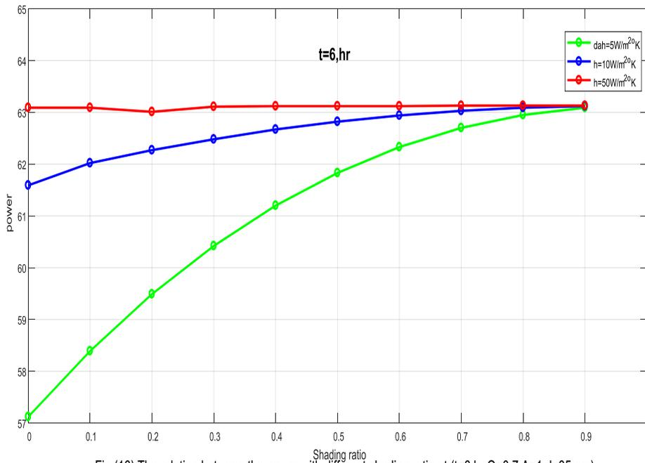
Fig.(16):The relation between the power with different shading ratio at:(t=6,hr,Q=0.7,A=1,d=35mm)
