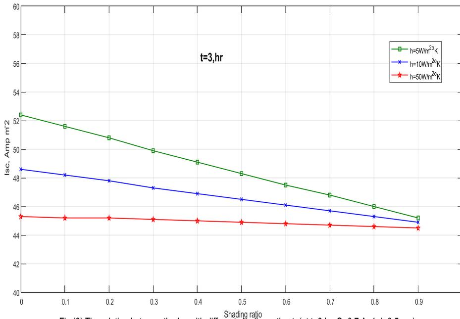
Fig.(9):The relation between the  $I_{sc}$  with different shading ratio at: (at  $t=3\text{hr}$ ,  $Q=0.7$ ,  $A=1$ ,  $d=3.5\text{mm}$ )
