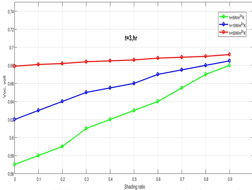
Fig.(12):The relation between the Voc with different shading ratio at:(t=3,hr,Q=0.7,A=1,d=35mm)
