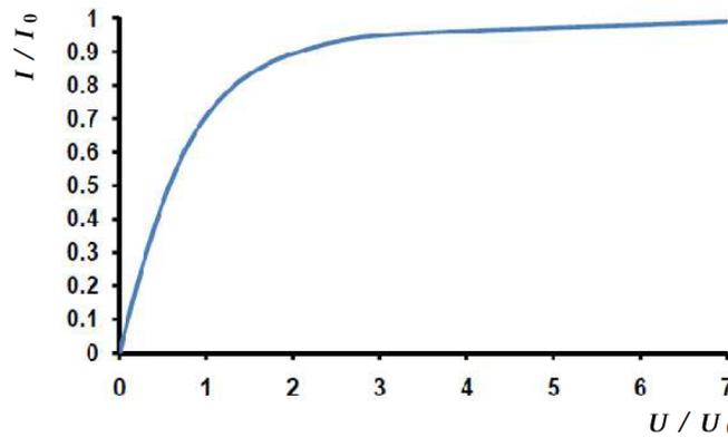
Figure 3: Current–voltage characteristics of 2D metal with hyperboloidal conduction band.
