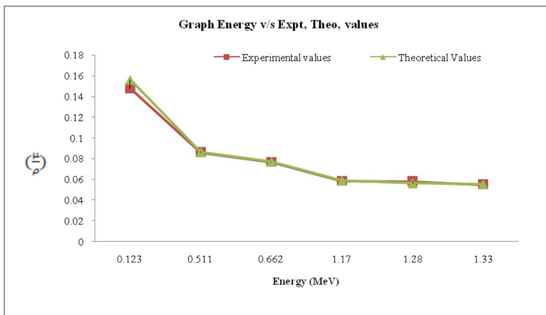
**Fig.3- Graph of Energy V/S experimental and Theoretical values of  $\left(\frac{\mu}{\rho}\right)$  for Magnesium Carbonate**
