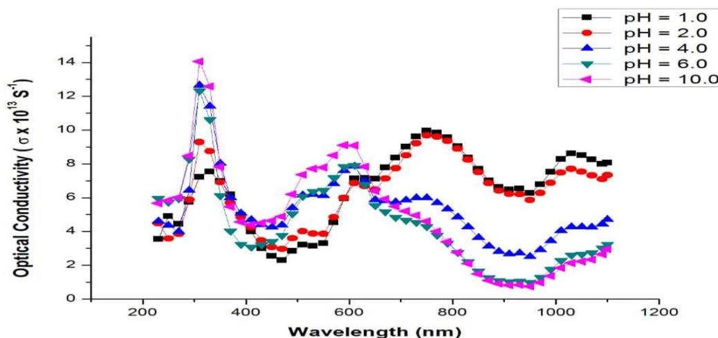
**Figure 7: Plot of optical conductivity versus wavelength PANI CMC samples at different pH variations**
