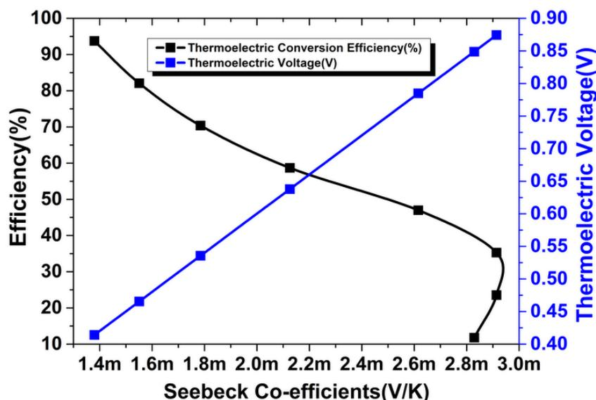
Fig.10: Thermoelectric voltage and conversion efficiency of  $\gamma$ -CuI versus Seebeck co-efficient.
