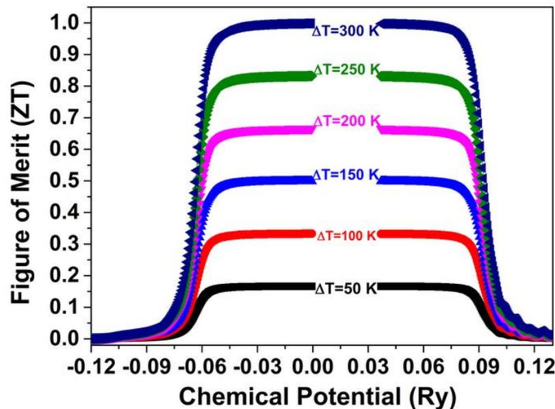
Fig.9: Variation of figure of merit with different temperature gradients.
