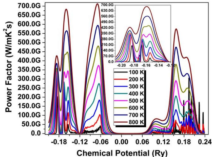
Fig.6: Thermoelectric power factor of  $\gamma$ -CuI for various temperatures.
