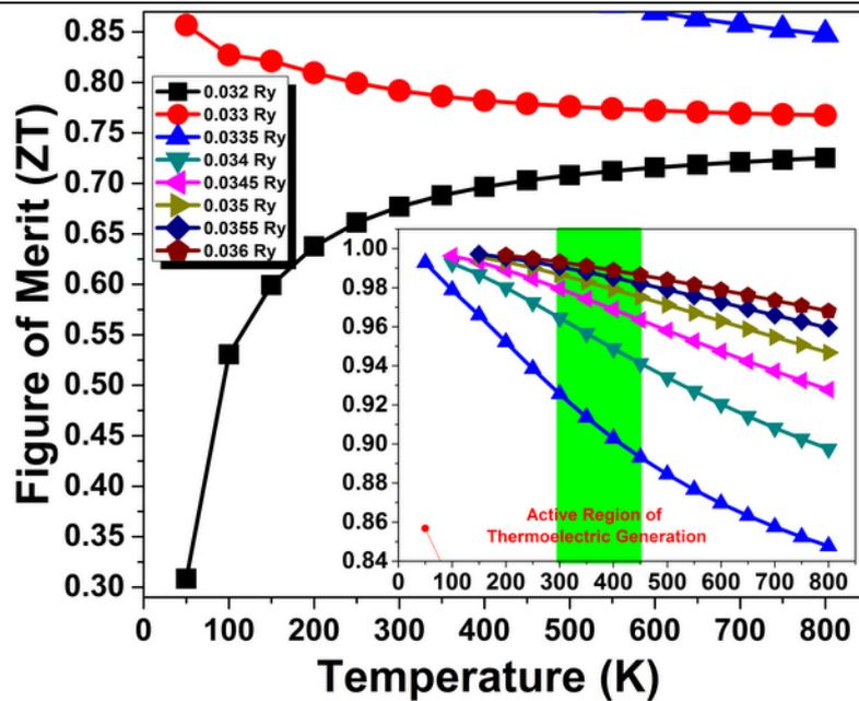
Fig.8: Variation of figure of merit versus temperature with optimum chemical potentials.
