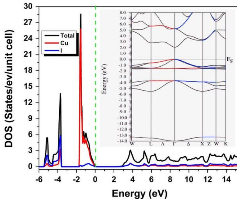
Fig.1: Density of states of  $\gamma$ -CuI, Inset: Band structure of  $\gamma$ -CuI.
