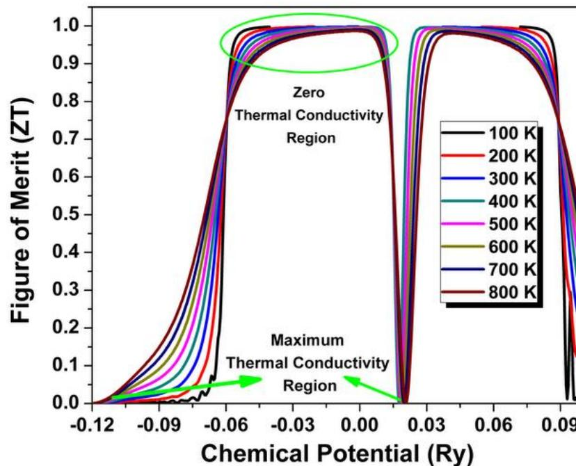
**Fig.7:** The calculated figure of merit versus chemical potential with various temperatures.
