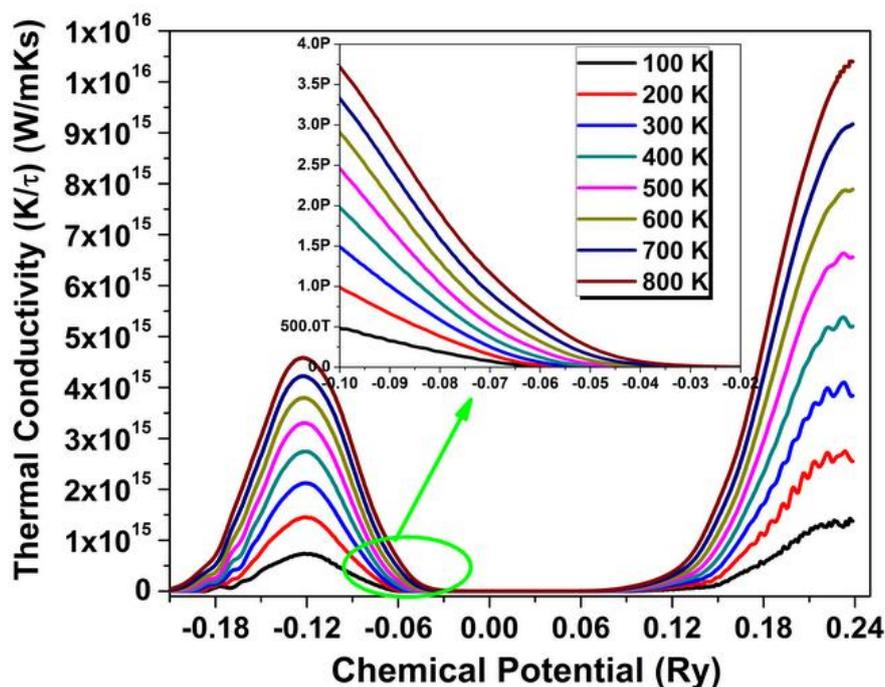
Fig.4: Thermal conductivity of  $\gamma$ -CuI versus chemical potential.
