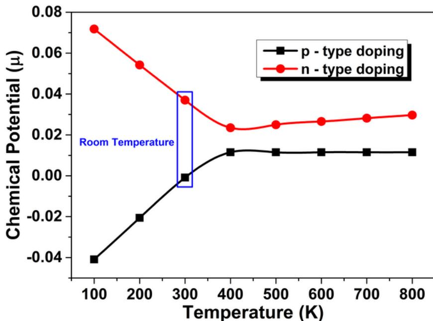
Fig.2: Chemical potential as a function of temperature.
