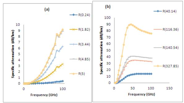
**4.10:** Results of Specific Attenuation for stratiform and convective
