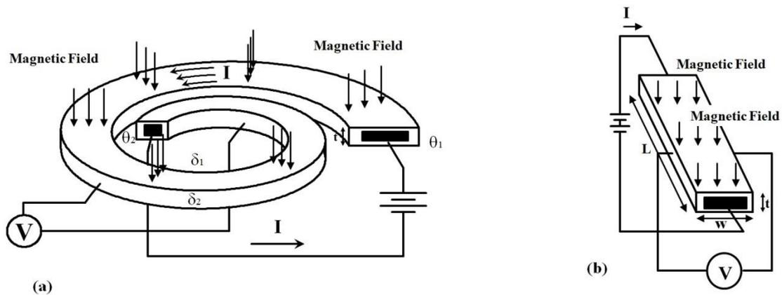
Figure 2. (a) The long spiral sheet and (b) the long rectangular sheet Hall concepts.
