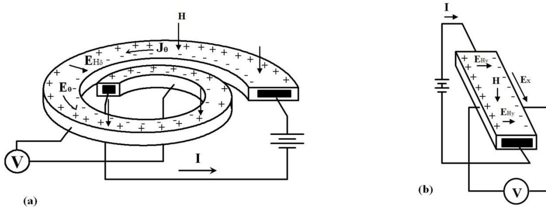
Figure 3: (a) The long spiral plate and (b) the long rectangular plate Hall voltage.
