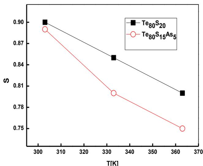
Fig [2] the exponent factor S as function of temperature T for the thin film samples  $Te_{80}S_{20}$  and  $Te_{80}S_{15}As_5$ .
