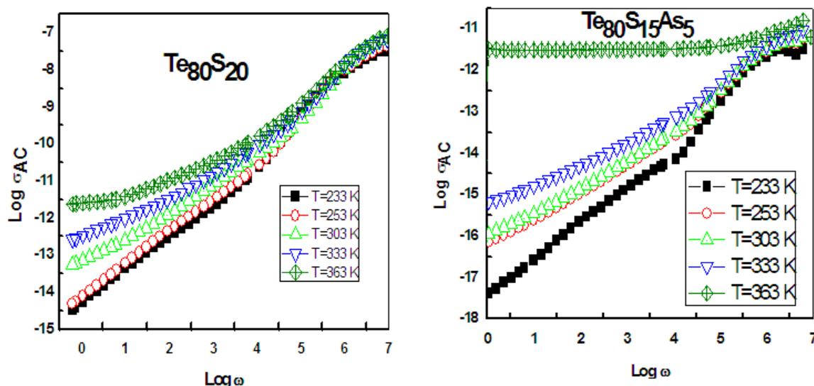
Fig [1] Variation of  $\text{Log } \sigma_{Ac}$  as a function of frequency at constant isotherms for the thin film samples  $Te_{80}S_{20}$  and  $Te_{80}S_{15}As_5$ .
