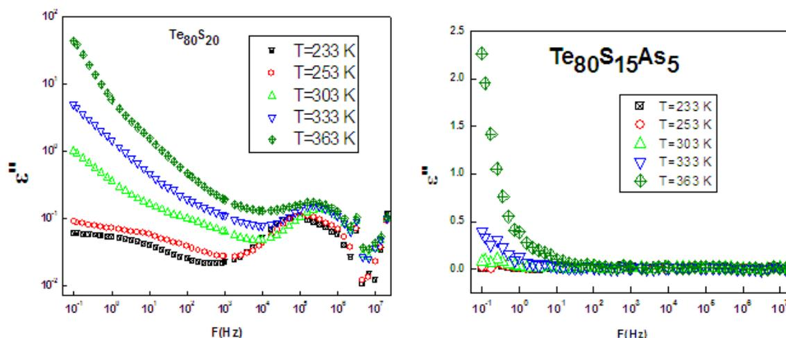
Fig [5] variation of the dielectric losses  $\epsilon''$  as function of frequency at different isotherms for the thin film samples  $Te_{80}S_{20}$  and  $Te_{80}S_{15}As_5$ .
