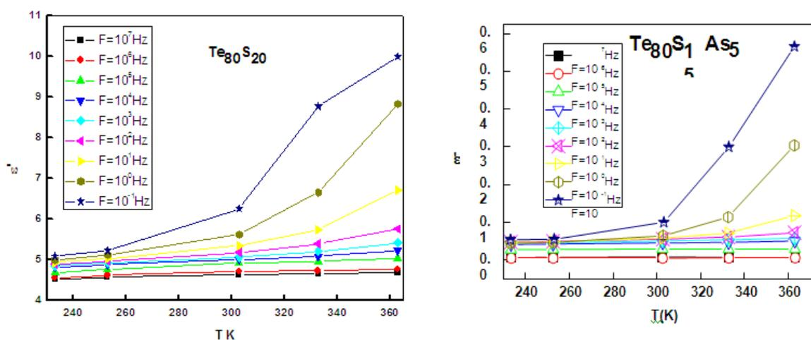
Fig [6] variation of dielectric constant  $\epsilon'$  as a function of temperature at different frequency for the thin film samples  $Te_{80}S_{20}$  and  $Te_{80}S_{15}As_5$
