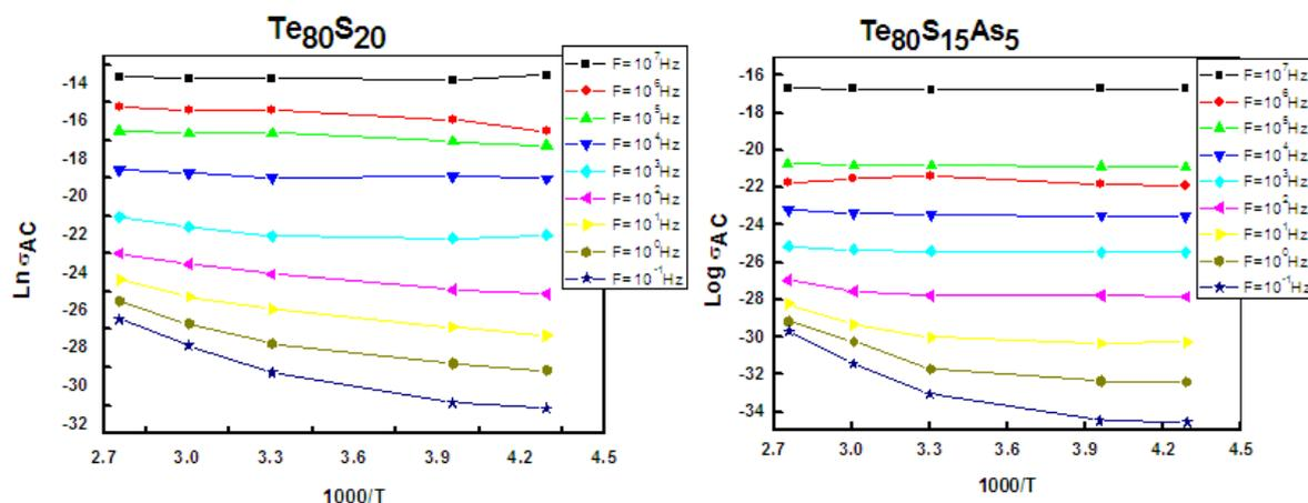
**Fig [3] Variation of  $\text{Ln } \sigma_{\text{Ac}}$  as function of  $1000/T$  at different constant frequencies for the thin film samples  $\text{Te}_{80}\text{S}_{20}$  and  $\text{Te}_{80}\text{S}_{15}\text{As}_5$  .**
