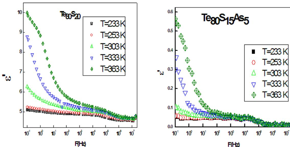
**Fig [4] variation of the dielectric constant  $\epsilon'$  as function of frequency at different isotherms for the thin film samples  $\text{Te}_{80}\text{S}_{20}$  and  $\text{Te}_{80}\text{S}_{15}\text{As}_5$  .**
