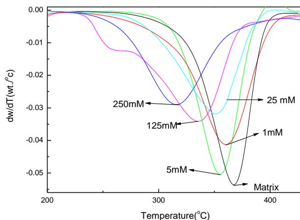
Fig.3 Derivative thermograms of matrix and the NCCFs prepared using 1 mM, 5 mM, 25 mM, 125 mM and 250 mM source solutions
