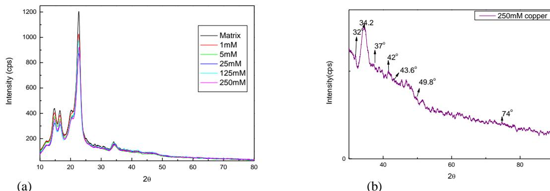
Fig. 2 X-ray diffractograms of the matrix and the NCCFs with in situ generated CuNPs using 1 mM, 5 mM, 25 mM, 125 mM and 250 mM source solutions (a) and Expanded diffractogram of the NCCF with in situ generated CuNPs using 250 mM source solution in  $2\theta = 35^\circ$  to  $80^\circ$  (b).
