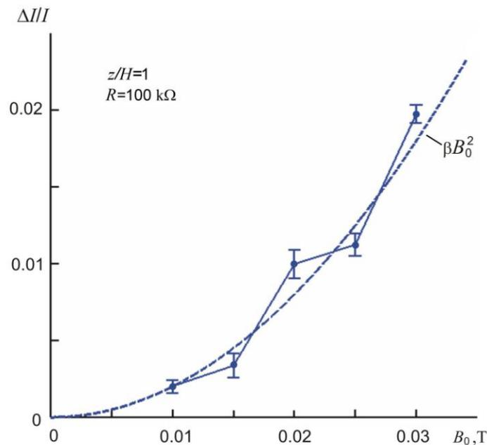
**Fig. 3. Relative change in current as a function of magnetic field induction.**
