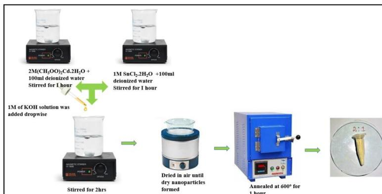
Fig.1. Graphical illustration for the synthesis of Cd<sub>2</sub>SnO<sub>4</sub> nanoparticles
