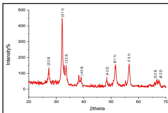
Fig. 2. Powder XRD pattern of the synthesized Cd<sub>2</sub>SnO<sub>4</sub> nanoparticles
