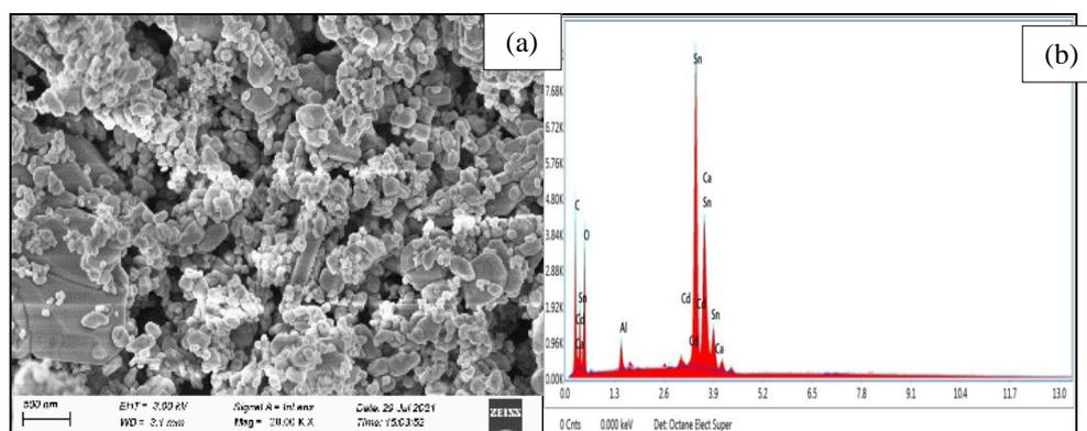
Fig.3.(a)FESEM imageand(b)EDX spectrum ofCd<sub>2</sub>SnO<sub>4</sub>nanoparticles.
