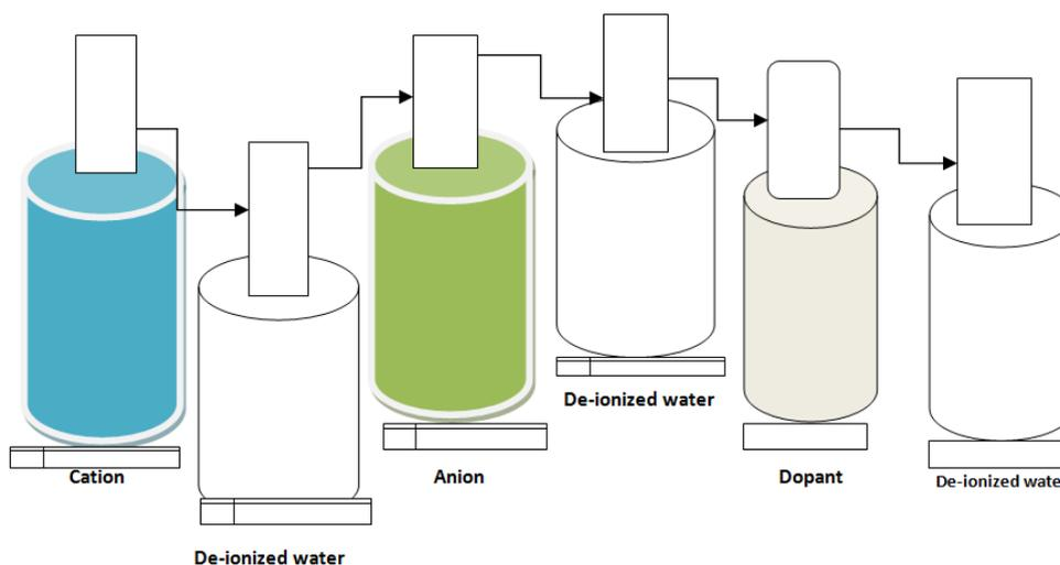
**Figure 1 The Setup of Advanced SILAR Deposition Process**
