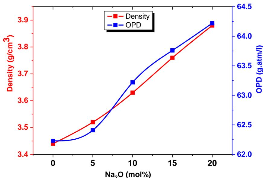
Fig 3. Variation of density and oxygen packing density with Na<sub>2</sub>O%.
