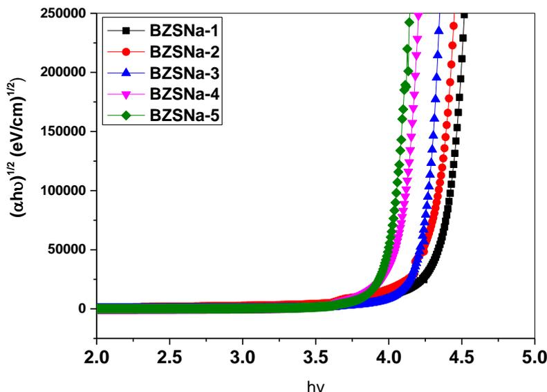
Fig. 5 Tauc plots for indirect band gap of BZSNa series
