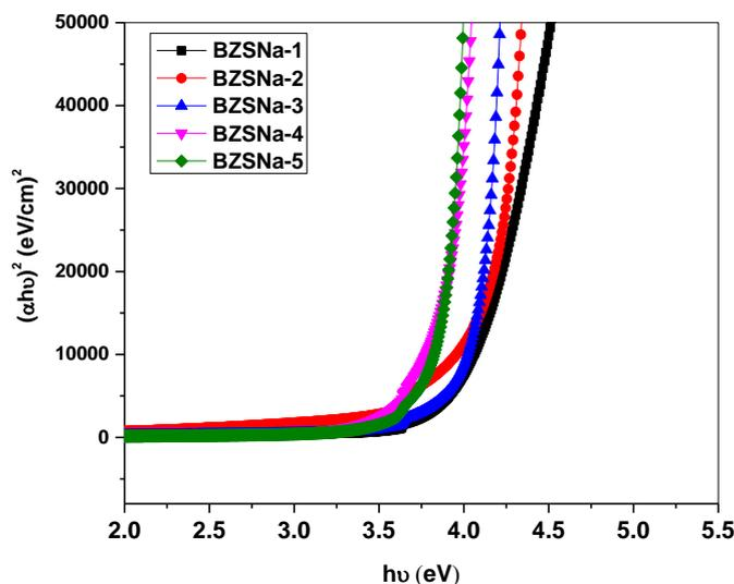
Fig. 6 Tauc plots for direct band gap of BZSNa series
