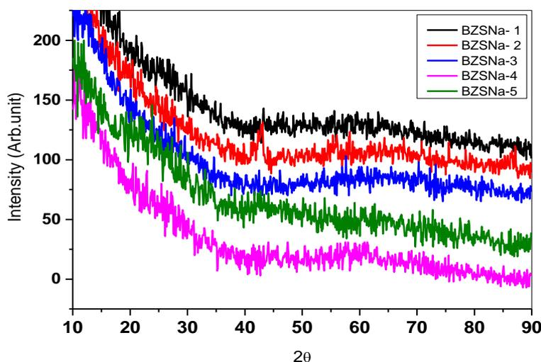
**Fig 1. XRD spectrograms of BZSNa glass system**
