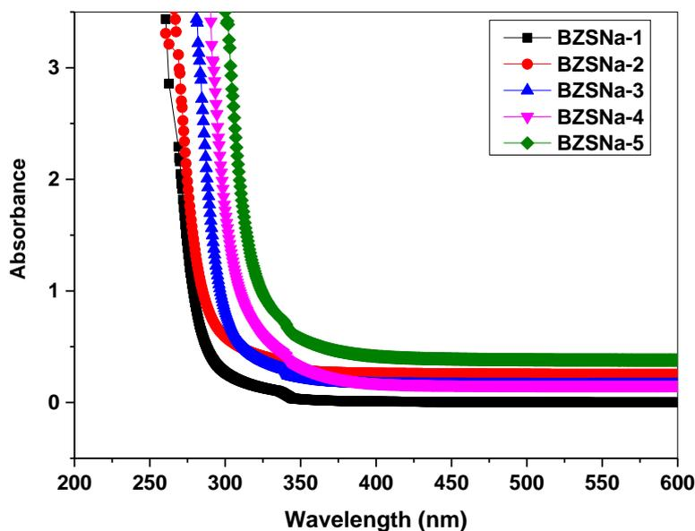
Fig. 4 Optical Absorption Spectra of BZSNa series
