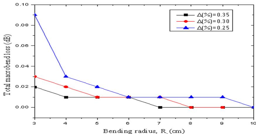
Figure 2: Total macro bend loss as a function of bending radius ( $R_c$ ).
