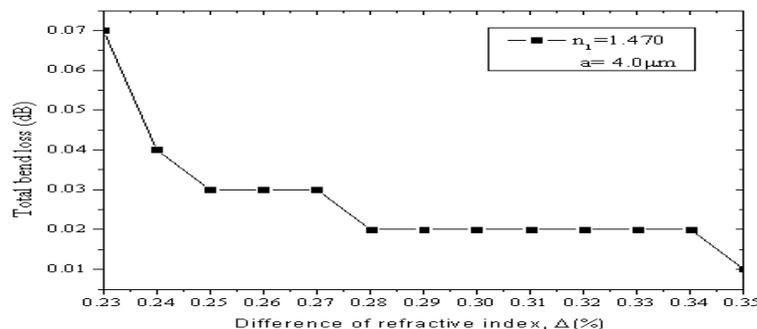
Figure 1: Total bend loss as a function of refractive index difference.
