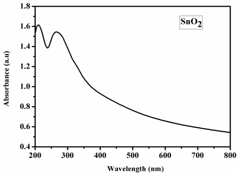
Fig. 3: UV-Vis absorption spectrum of SnO<sub>2</sub> NPs
