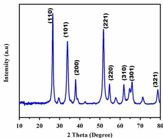
Fig. 1: XRD spectrum of  $\text{SnO}_2$  NPs
