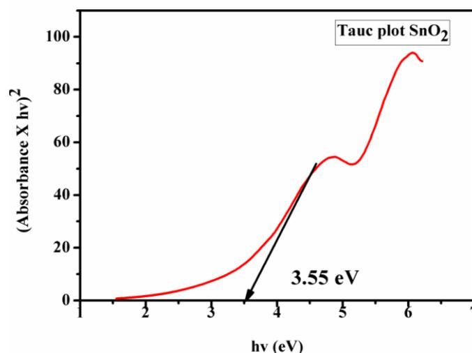
Fig. 4: Tauc plot of SnO<sub>2</sub> NPs
