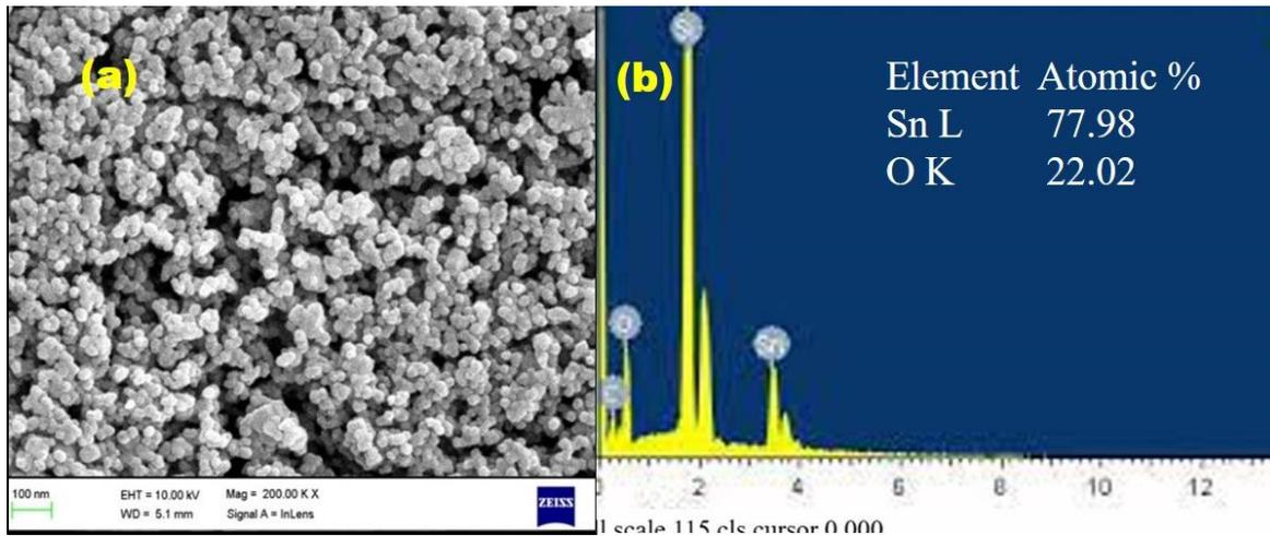
Fig. 2: (a) SEM image (b) EDX spectrum of SnO<sub>2</sub> NPs
