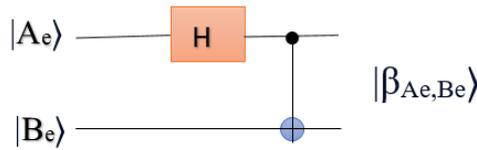
**Figure 2:** Quantum Circuit for generating Bell states consists of a Hadamard Gate (the orange box H) and a CNOT Gate (the purple circle with a plus sign inside it, signifying the XOR operation). The input qubits are  $|A_e\rangle$  and  $|B_e\rangle$  and the output state is a maximally entangled state  $|\beta_{A_e, B_e}\rangle$ .
