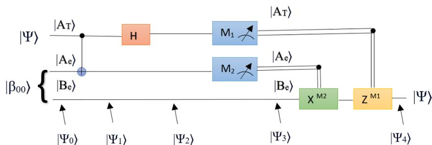
**Figure 1:** Quantum Circuit showing three qubit system (three single lines), with upper two qubits ( $|A_T\rangle$  and  $|A_e\rangle$ ) correspond to Alice and the third ( $|B_e\rangle$ ) corresponds to Bob. The double lines show classical wires, the rectangular boxes represent Hadamard Gate (orange box), measurement instruments ( $M_1$  and  $M_2$  in blue boxes), Pauli's X-Gate (green box), and the Pauli's Z-Gate (yellow box). The purple circle represents the CNOT gate.
