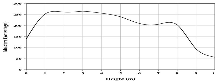
Fig. 7. The total moisture content (gm) inside the control volume for heights from 0 to 10 m
