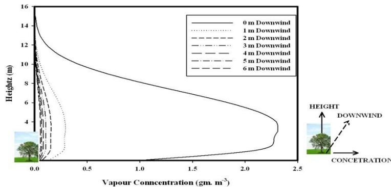
Fig. 3. Concentration profiles downwind showing variation with height.
