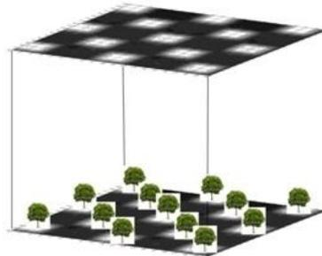
Fig. 1. A control volume with moisture concentration at two planes of observation at the base  $z=0$  and top  $z=h_{cv}$
