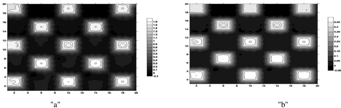
Fig. 6. Contour plot of moisture concentration for the control volume at tow height a:z=7, b: z= 10 m
