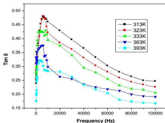
Figure 9. Variation of loss tangent with frequency
