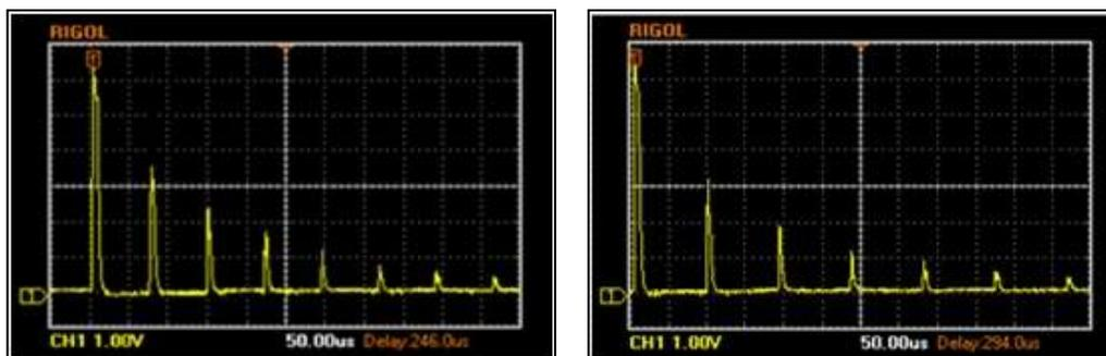
Fig. 6(b): Echo pattern for *ethanol* at 5MHz for path length of 35.0 mm and 45.0 mm respectively.
