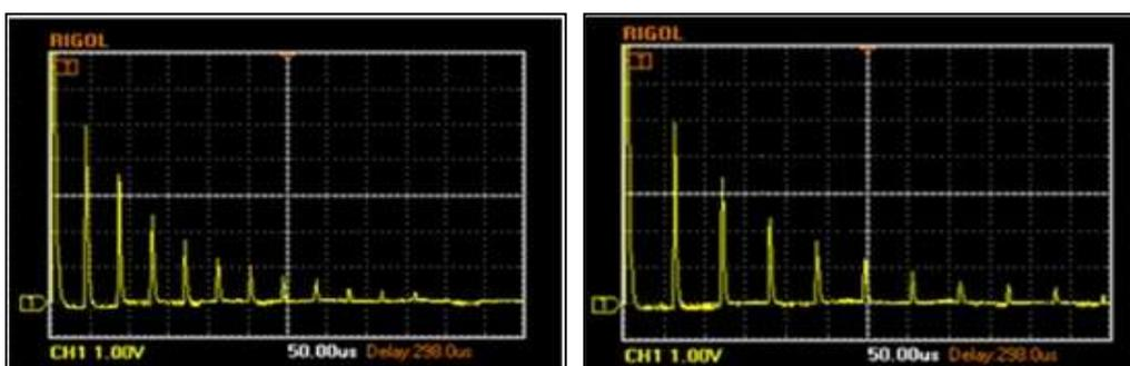
Fig. 5(b): Echo pattern for *acetone* at 5MHz for path length of 20.0 mm and 30.0 mm respectively
