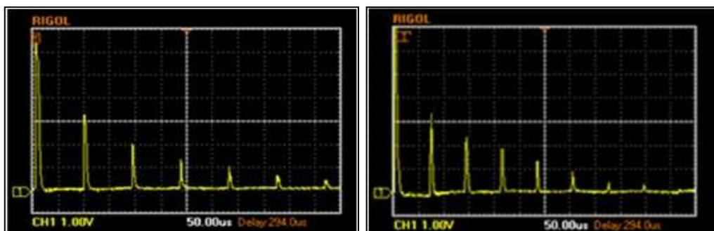
Fig. 6(a): Echo pattern for *ethanol* at 2MHz for path length of 41.3 mm and 51.3 mm respectively.
