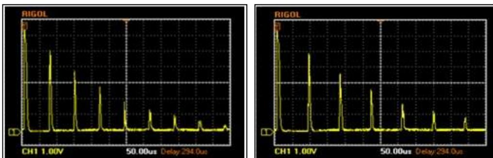
Fig. 5(a): Echo pattern for *acetone* at 2MHz for path length of 41.3 mm and 51.3 mm respectively
