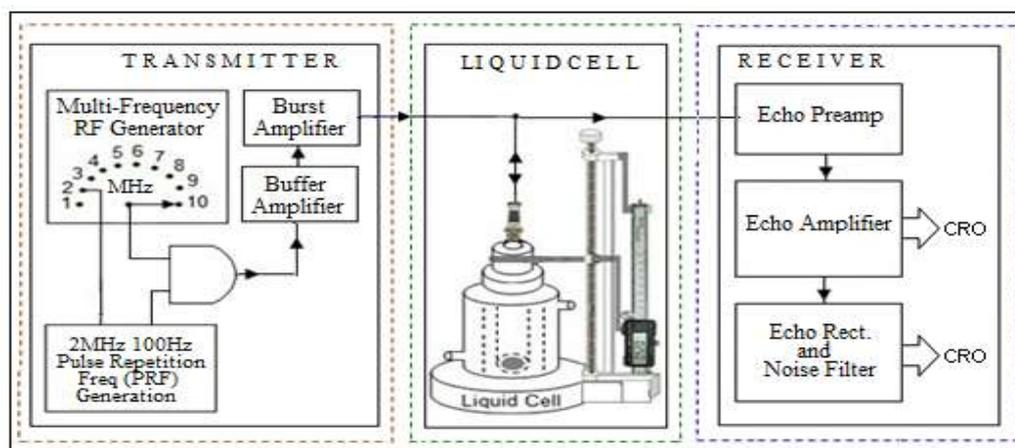
Fig. 2: Block diagram of Multi-Frequency Ultrasonic Pulse-Echo System
