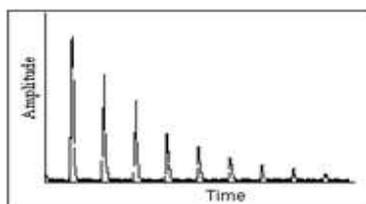
Fig. 1: Typical pulse-echo decay pattern
