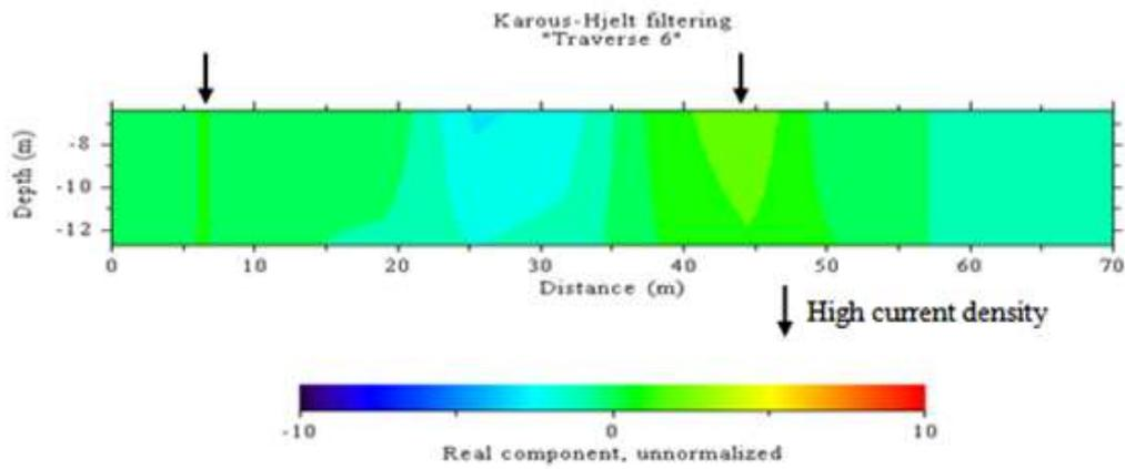
Figure 8: Karous-Hjelt current density plots for VLF-em profile 4
