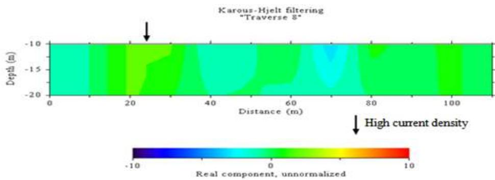
Figure 9: Karous-Hjelt current density plots for VLF-em profile 5
