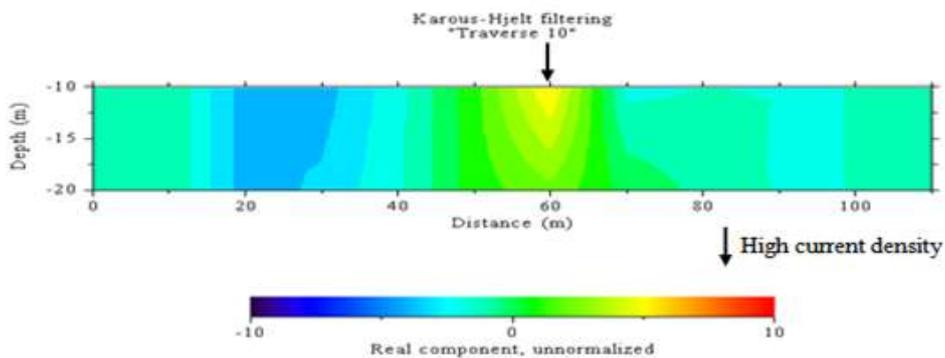
Figure 11: Karous-Hjelt current density plots for VLF-em profile 7
