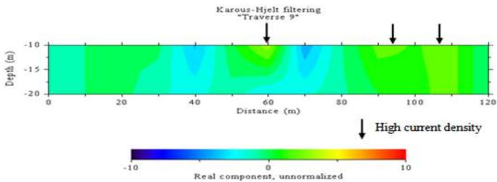
Figure 10: Karous-Hjelt current density plots for VLF-em profile 6
