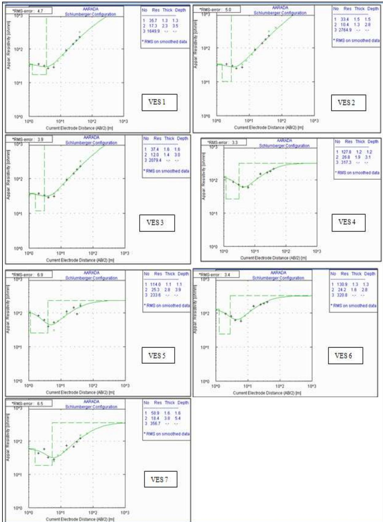
Figure 13: The model curves for VES 1 to VES 7
