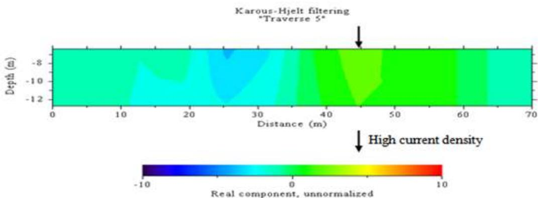
Figure 7: Karous-Hjelt current density plots for VLF-em profile 3
