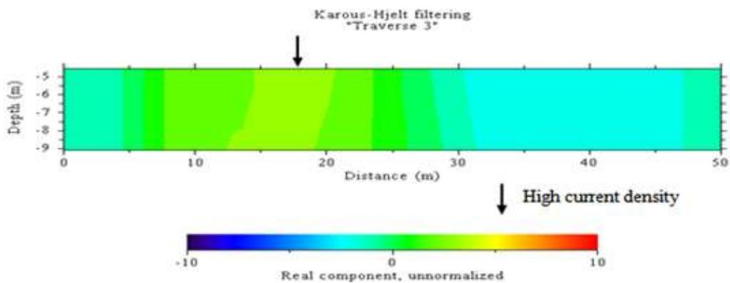
Figure 5: Karous-Hjelt current density plots for VLF-em profile 1
