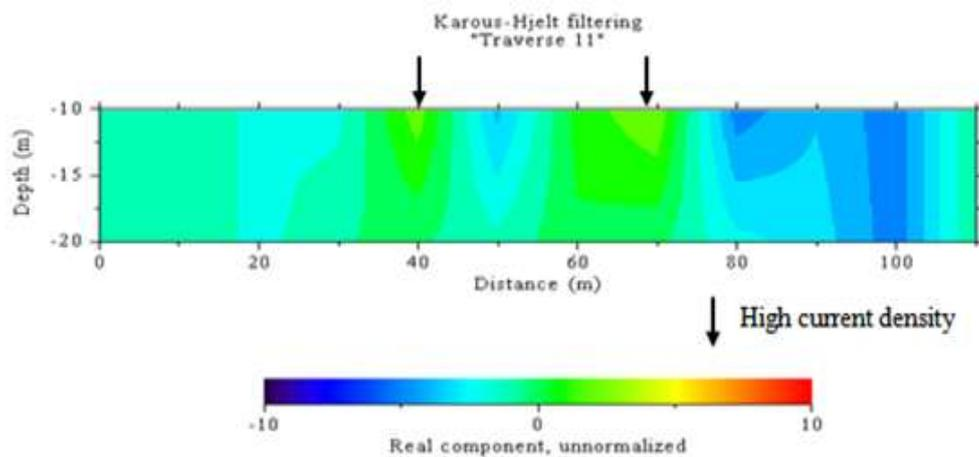
Figure 12: Karous-Hjelt current density plots for VLF-em profile 8
