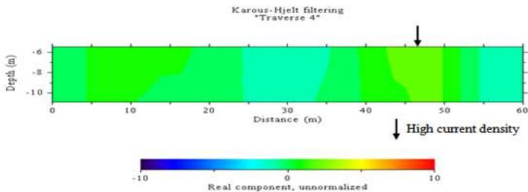
Figure 6: Karous-Hjelt current density plots for VLF-em profile 2
