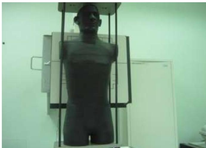
**Figure 1 The Rando man phantom used in present investigations Phantom dosimetry procedures**
