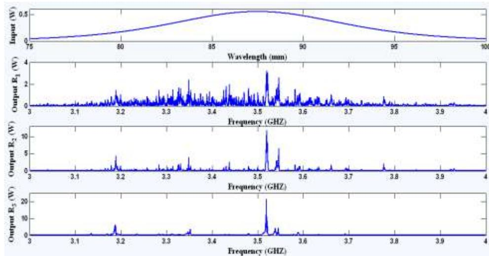
**Fig. 2:** Results obtained when frequency soliton pulse is localized within a microring device with 20,000 roundtrips, the ring radii are  $R_1= 10\ \mu\text{m}$  ,  $R_2= 10\ \mu\text{m}$  ,  $R_3= 12\ \mu\text{m}$
