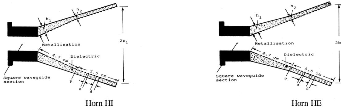
Fig.1. E-Plane view of the horn HI with interior throat tapering profile, horn HE with exterior throat tapering profile and their design details.
