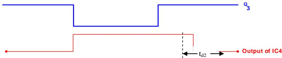
Fig. 6 Waveforms of the outputs of Q3 and IC4
