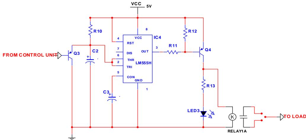
Fig. 5 Schematic diagram of the time delay unit and the switching unit
