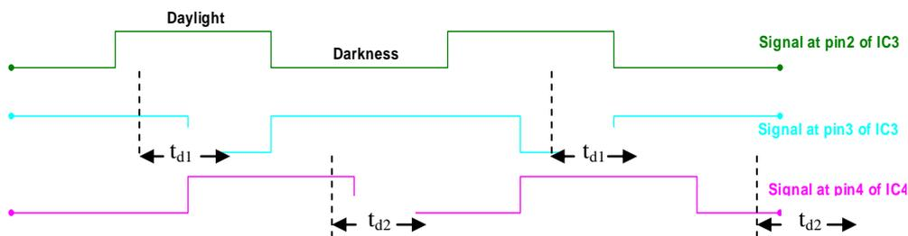
Fig. 7 Waveforms summarizing the flow signals of the system
