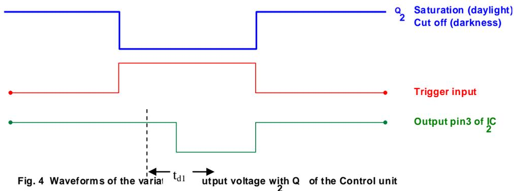
Fig. 4 Waveforms of the variable output voltage with  $Q_2$  of the Control unit
