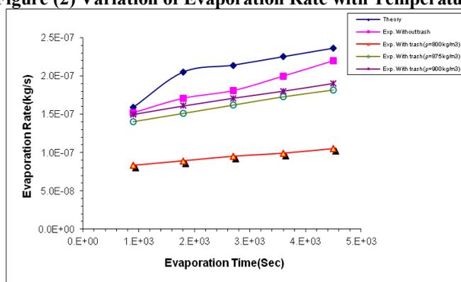
Figure (3) Variation of Evaporation Rate with Time
