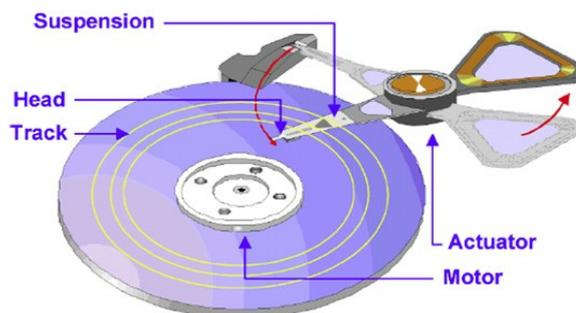
**Fig.8.** Schematic diagram of a hard disk platter showing recorded tracks, actuator and suspension onto which the head is attached. [32].
