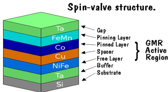
Fig.7. Spin Valves Sensors
